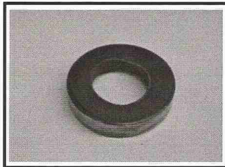
26] PUSH THE NEW GLAND INTO THE RETAINER.
